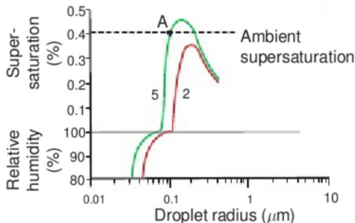
**Fig. 6.4** Köhler curves 2 and 5 from Fig. 6.3. Curve 2 is for a solution droplet containing  $10^{-19}$  kg of NaCl, and curve 5 is for a solution droplet containing  $10^{-19}$  kg of  $(\text{NH}_4)_2\text{SO}_4$ . The dashed line is an assumed ambient supersaturation discussed in the text.
