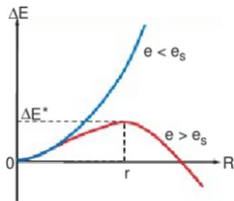
**Fig. 6.1** Increase  $\Delta E$  in the energy of a system due to the formation of a water droplet of radius  $R$  from water vapor with pressure  $e$ ;  $e_s$  is the saturation vapor pressure with respect to a plane surface of water at the temperature of the system.
